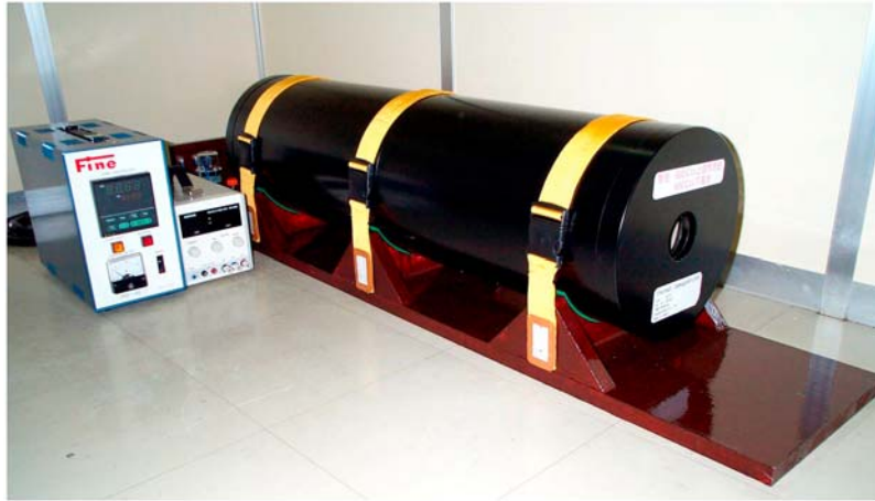
Figure 3. Newly constructed Sogo Fine-TD thermal demagnetizer. With accuracy of temperature control and reproducibility to less than 1°C and with an extraordinarily low AC field ( \sim 2 \mu\text{T} ) inside the oven during heating, this thermal demagnetizer enables very high resolution investigations of paleomagnetism and rock magnetism on rocks.
